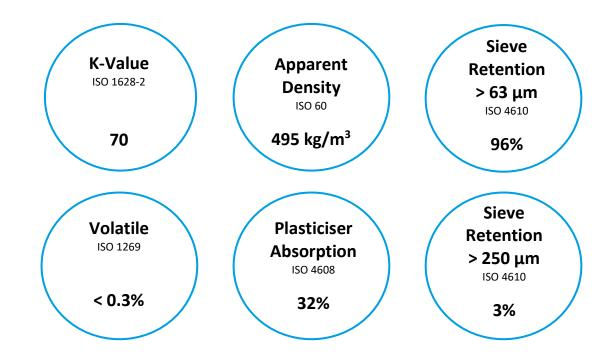
Note: The property data shown above has been obtained from laboratory tests on representative samples of VYNOVA<sup>TM</sup> S7102 polymer. Although the values are typical, they are for guidance only, and must not be used as a basis for specifications.
