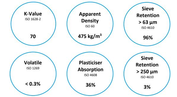
Note: The property data shown above has been obtained from laboratory tests on representative samples of VYNOVA<sup>™</sup> S7000 polymer. Although the values are typical, they are for guidance only, and must not be used as a basis for specifications.
